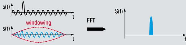
The R&S®RTE overlaps the FFT, captures small pulse peaks and uses color-coding to display them
