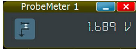
R&S®ProbeMeter: high DC measurement accuracy, independent of the instrument settings and in parallel with the measurement channel.
