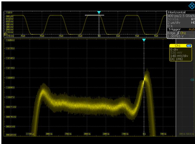
The high sensitivity of the Rohde&Schwarz digital trigger makes it possible to trigger on signal overshoots of less than 9 mV, as can be seen in the example below. At a vertical scale of 140 mV/div, this corresponds to only a fraction of one display division.
