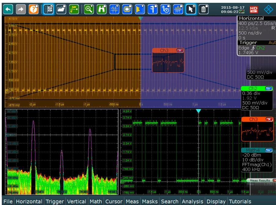
The user can drag & drop waveforms and result windows on the screen. The Rohde & Schwarz SmartGrid function helps users arrange multiple diagrams or tabs on the screen. The size of individual diagrams can be further optimized by dragging the edges of the windows.
